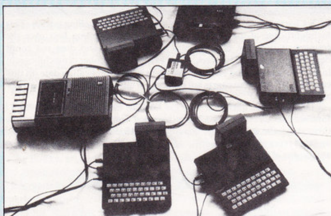
NEAT NETS — Home computers including the ZX81, Spectrum, BBC, Dragon and Jupiter Ace can be tied into the Multiload, which could be a cheap introduction to networking. A network for four home computers costs £7.98 and lets you transmit programs, data and screen content from one device to the others, while multi-saving lets one computer record onto various tape players simultaneously. The product is available now from Network Computer Systems on Luton (0582) 508616.
