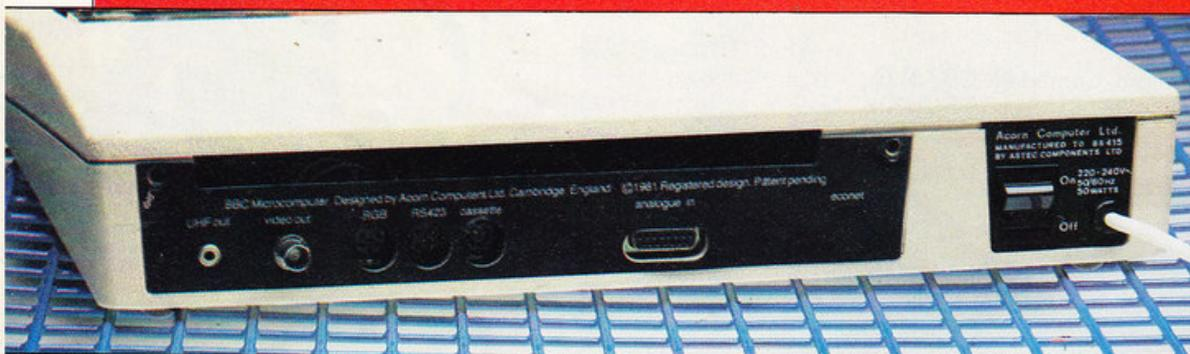
Left is the rear of the casing with connections for video output, RS432 port, cassette output and analogue input.
