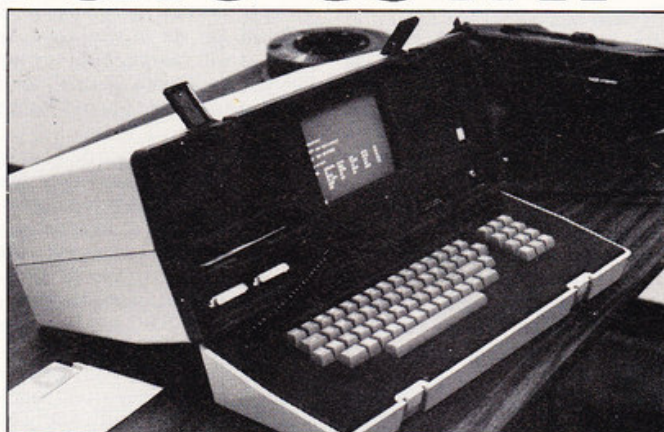
Adam Osborne marked his visit to London by launching the Executive. Selling at £1995 plus VAT, it is a major improvement on the old Osborne 1 with a 7in amber display, double density disk drives holding 200K per disk, CP/M+ and UCSD-p operating systems as added features. And to round up the package £2,000 worth software is thrown in ( PCN , Issue 8).
