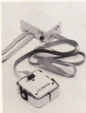
★ Compact and rugged mobile robot, 5½ x 5 x 2" with two DC motor drive.
