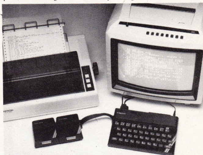
The Microdrive Interface 1 includes an RS232 interface allowing connection with peripherals such as high quality printers.
