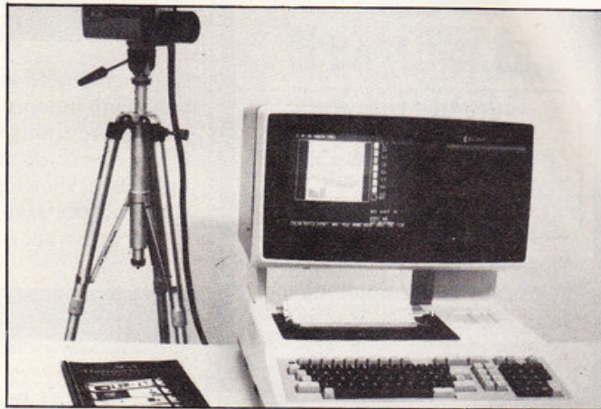
BMC if800 thermal analysis system model 30, as used by Aga Infrared.
