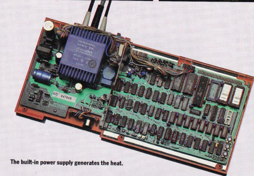
The built-in power supply generates the heat.
