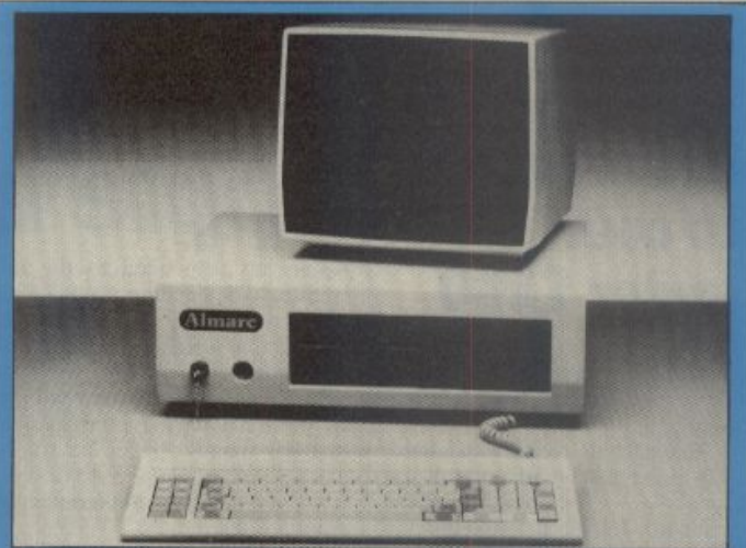
SPIRIT — This expensive looking micro, comprising what looks like an IBM keyboard and repainted Sirius cabinet, actually contains the powerful Motorola 68000 16-bit microprocessor. The machine is part of the Almarc Data Systems Spirit range of micros which now offers a choice of 280, 8086 and 68000 processors. The 68000 version can run the multi-user operating system Unix and you get 10Mb of Winchester disk storage as an extra bonus. Almarc claims the Spirit 1-68 is ready for delivery in exchange for £4,000 plus VAT. The company is on 0602-52657.
