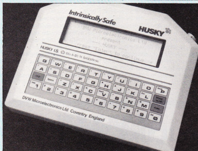
WARM AND HUSKY — DVW Microelectronics has repackaged its Husky portable to make it suitable for anyone using a micro in what it describes as 'flammable or explosive atmospheres'. The new model is known as the Husky IS (Intrinsically Safe). The Z80-based machine with 128 character LCD will sell from £2,099 for a 16K version to £3,144 for the 144K version. DVW is on Coventry (0203) 668181.
