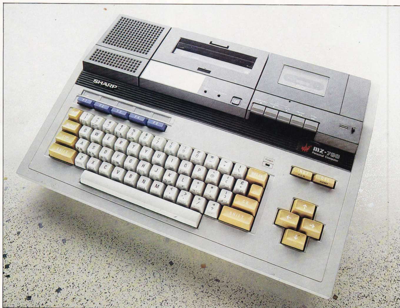
The front of the Sharp MZ 731 (above) shows the keyboard layout and the integrated speaker, plotter and cassette deck from left to right across the top. The close-up of the cassette deck (right) shows how compact it is, despite its taking standard audio cassettes. Below it can be seen the insert and delete keys and the power light.
