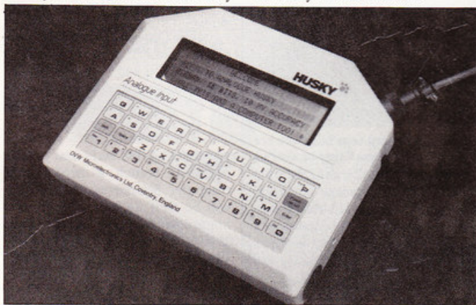
Husky equipped with analogue input.
