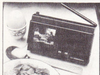
Sinclair's flat-screen TV uses a single integrated circuit chip to perform the majority of signal processing functions. The £79.95 2in TV is the first television to have all such functions controlled by a single chip.
