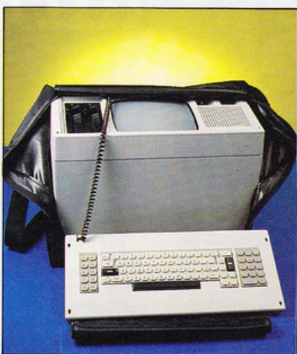
Top: The Miracle is a good looking all-in-one unit weighing 28lbs. Right: A shoulder bag is provided to allow you to carry the otherwise immobile machine.
