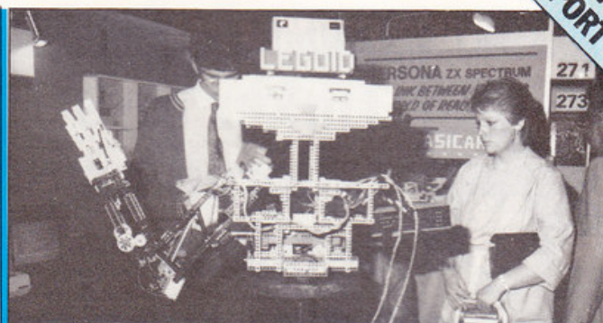
LEGO POWER — Basicare Microsystem has injected life into Lego. Driven by a Spectrum and using an interface developed by the company, the robot is able to move round freely under its own steam. This robot is one of many projects which the company has undertaken to show how a micro can control processes in the real world. It isn't for sale, though.
