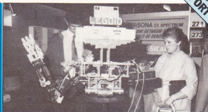
LEGO POWER — Basicare Microsystem has injected life into Lego. Driven by a Spectrum and using an interface developed by the company, the robot is able to move round freely under its own steam. This robot is one of many projects which the company has undertaken to show how a micro can control processes in the real world. It isn't for sale, though.
