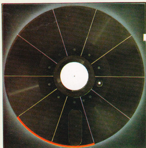
The Acorn DFS allocates two sectors on track 0 of the floppy disk for the directory, giving you 31 files.
