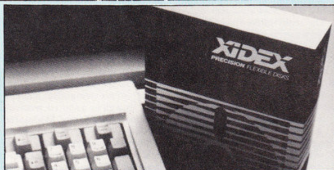
MAGNETIC FLOPPIES — Another addition to the mass of floppy disks on the market is Xidex's new line of 5¼in and 8in Precision flexible disks. With 96 tracks per inch the disks are made of the latest magnetic materials, the company says. To reduce head-to-disk interchange problems due to shifting of the disk in the drive, Xidex has improved the tolerance on the inside diameter of the disk's centre hole by fifty per cent. Contact BFI, 01-941 4066.
