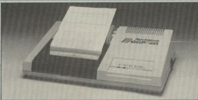
COLOUR SCHEME — Newly arrived from Japan is this four-colour printer-plotter for £129.95. Distributed by Micro Peripherals, the MCP-40 (nothing to do with pigs) works on any micro with a parallel interface. Producing up to 80 characters per line at 12 characters per second, it plots charts or graphs in four colours. Also out is its little brother, the MP-24, which sells for £86.25. This 24-column printer runs at 42 lines a minute, comes with ribbon, cable, and plug and also works on micros with parallel interfaces. More information from Micro Peripherals in Basingstoke on 0256 3322.
