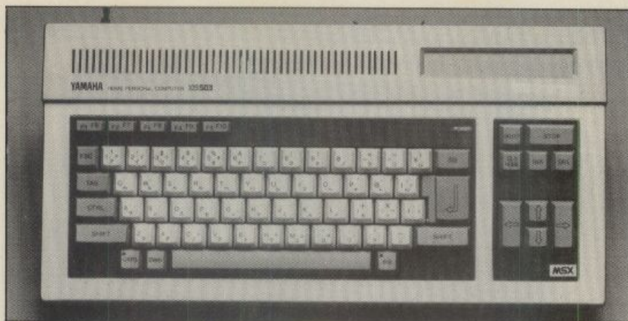
The Yamaha keyboard has a nice feel — the layout is standardised by the MSX conventions. The beloved diamond arrangement of the cursor keys has been substituted with a square.
