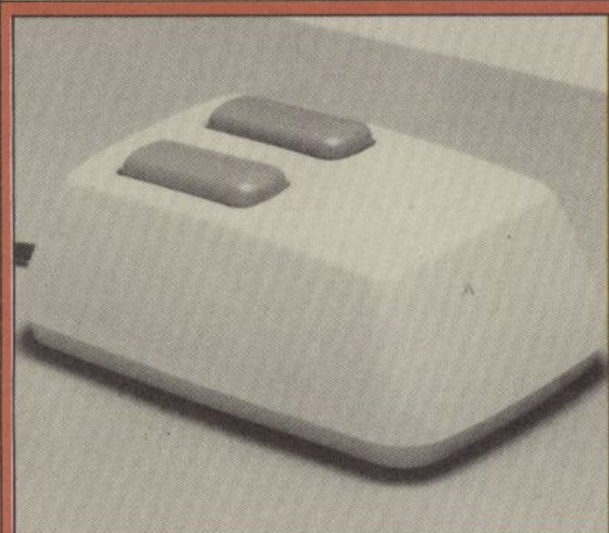
MOUSE DANCE — Disk maker Shugart has branched out into the rodent business by producing a mouse with no moving parts. This makes it an optical mouse, according to the jargon that is growing up around such devices. The main advantage is that it doesn't need the regular check-ups that punctuate the working lives of other mice, and Shugart says it's lighter and quieter into the bargain. Other fascinating details — you can move the device at 25ins a second and buy it in two- or three-button versions.
