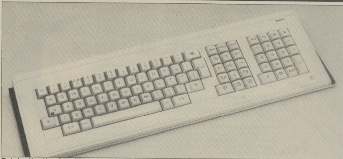
The keyboard layout has a Super shift key and two control keys, guarding the space bar.
