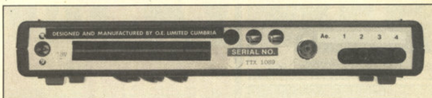
The TTX2000 in all its glory. Tuning knobs, aerial socket and power supply are at the back.
