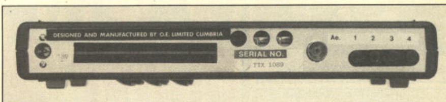
The TTX2000 in all its glory. Tuning knobs, aerial socket and power supply are at the back.
