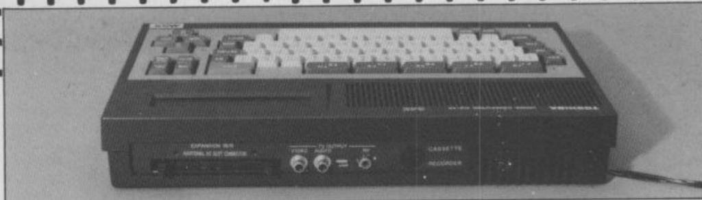
Rear view of HX-10 showing connector ports.
