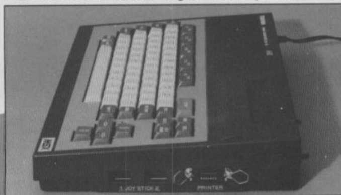
Side view of HX-10 showing connector ports.
