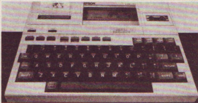
Epson's HX-20 portable micro has 16K Ram and a 20X4 liquid crystal display.
