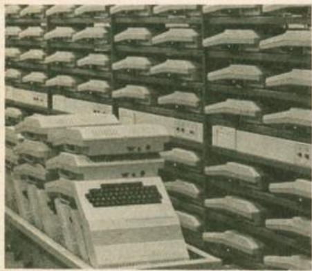
Twenty-four-hour soak-testing.
