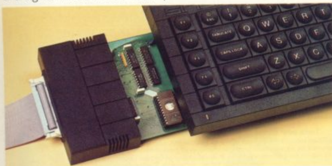
A Centronics interface slips discreetly into place.
