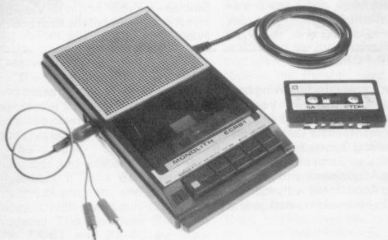
A cassette recorder developed for the ZX-81.
