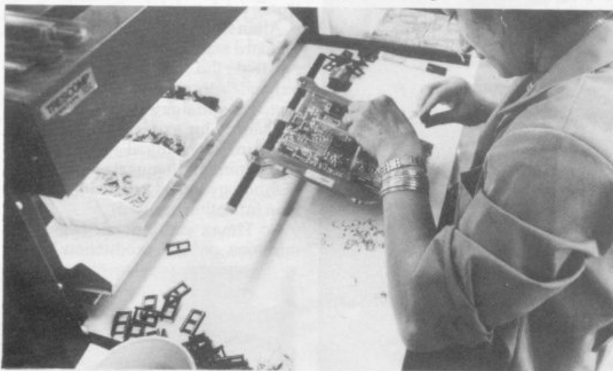
Building up the circuit board
