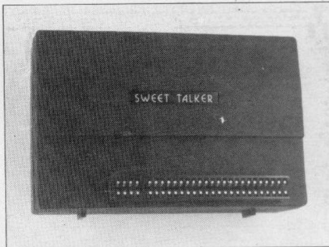
allow you to produce the sounds necessary to make up a full word. They are put out as numbers to Sweet Talker in sequence from a DATA statement when you want words spoken. Silences can be included to stop the words or to provide pauses between words — of up to 200ms. The Sweet Talker seems to be
