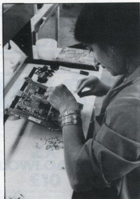
Building-up the circuit board
