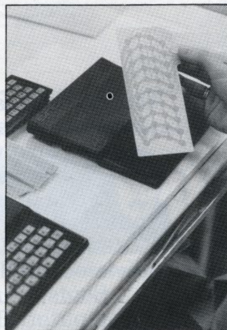
Assembling the keyboard
