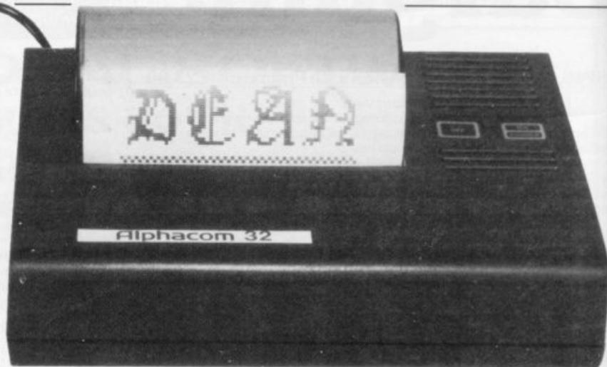
This thermal printer, now available in the U.K., is the standard printer used with the American version of the ZX81. The printer plugs direct into the Spectrum but has a through port allowing the use of additional hardware through the same connector.
