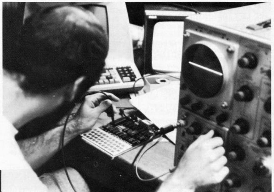
Photo 6 Trying to locate the reversed diodes
