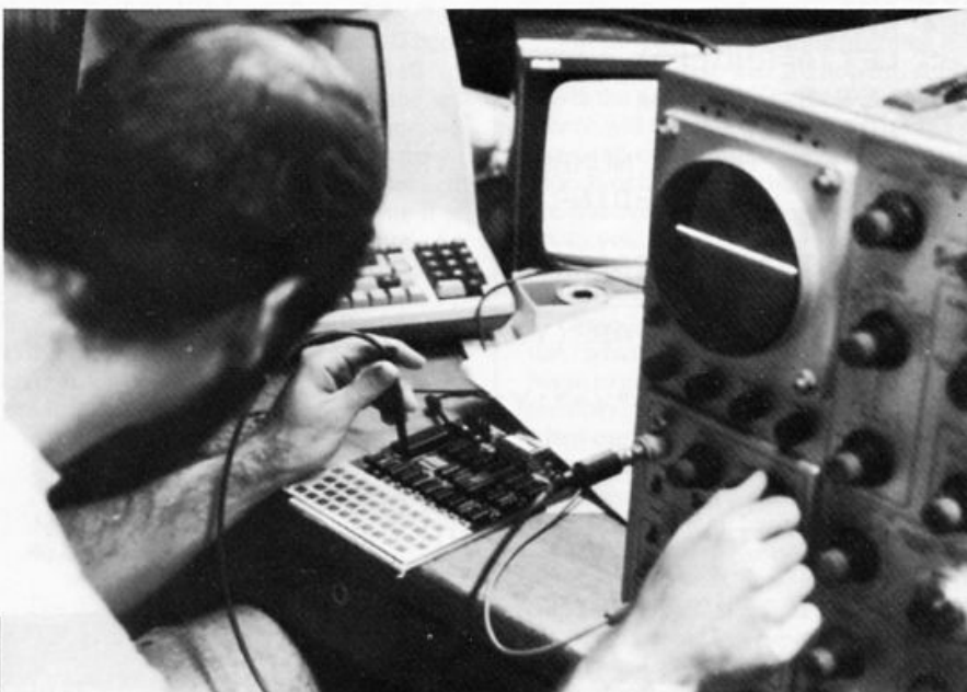
Photo 6 Trying to locate the reversed diodes
