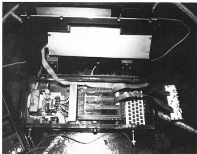
Figure 5. The inside of the author's system. The parallel interface and extra memory are located on the expansion board mounted above the computer.
