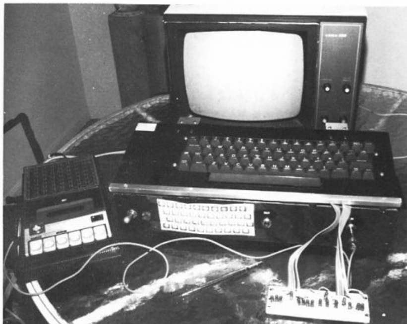
Figure 4. Author's 8K MicroAce system connected to a standard video monitor and standard size keyboard. The bread board in the foreground holds 16 LEDs which are used to monitor the outputs of both ports.
