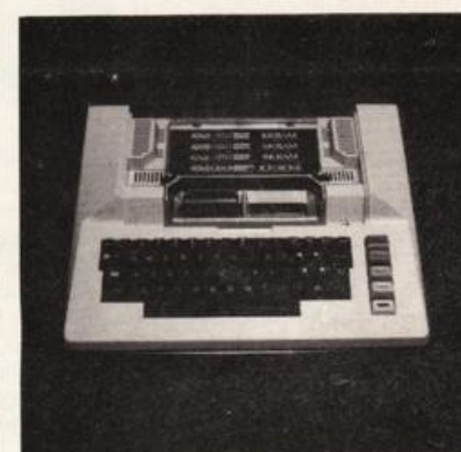
Atari 800 Console (with cover removed)
