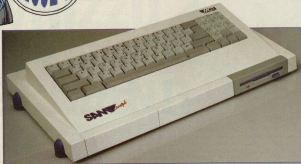
The Coupé's slot-in disk drive
