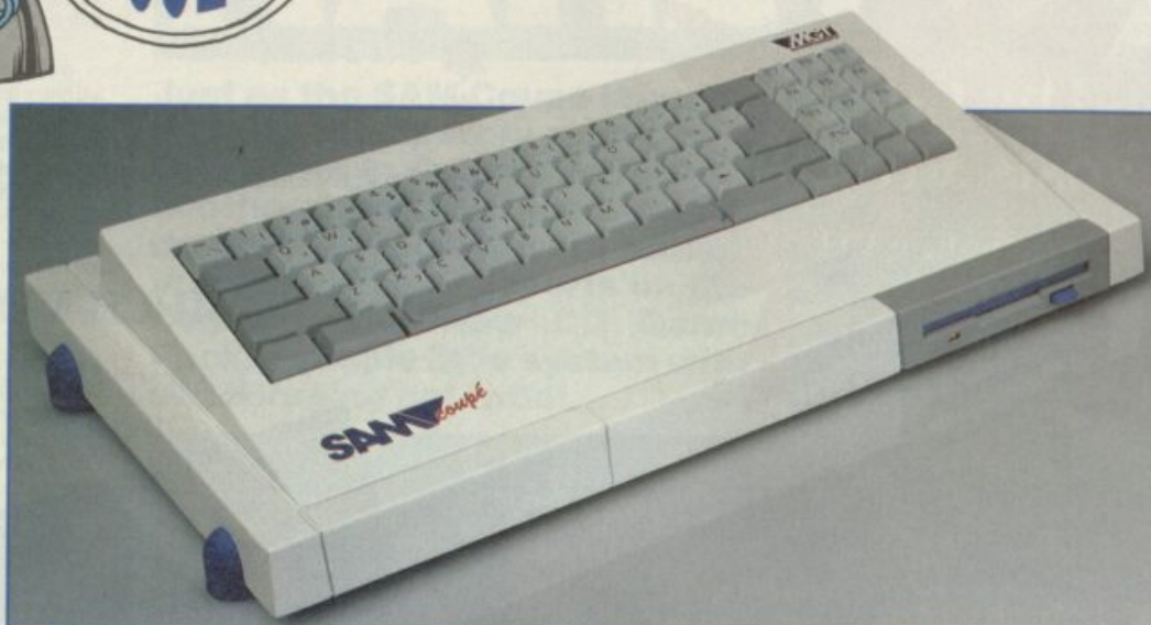
The Coupé's slot-in disk drive
