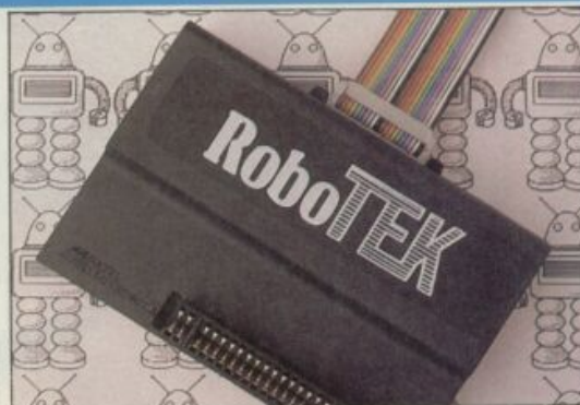
With a Robotek interface you can use the Spectrum to control a robot's movements.
