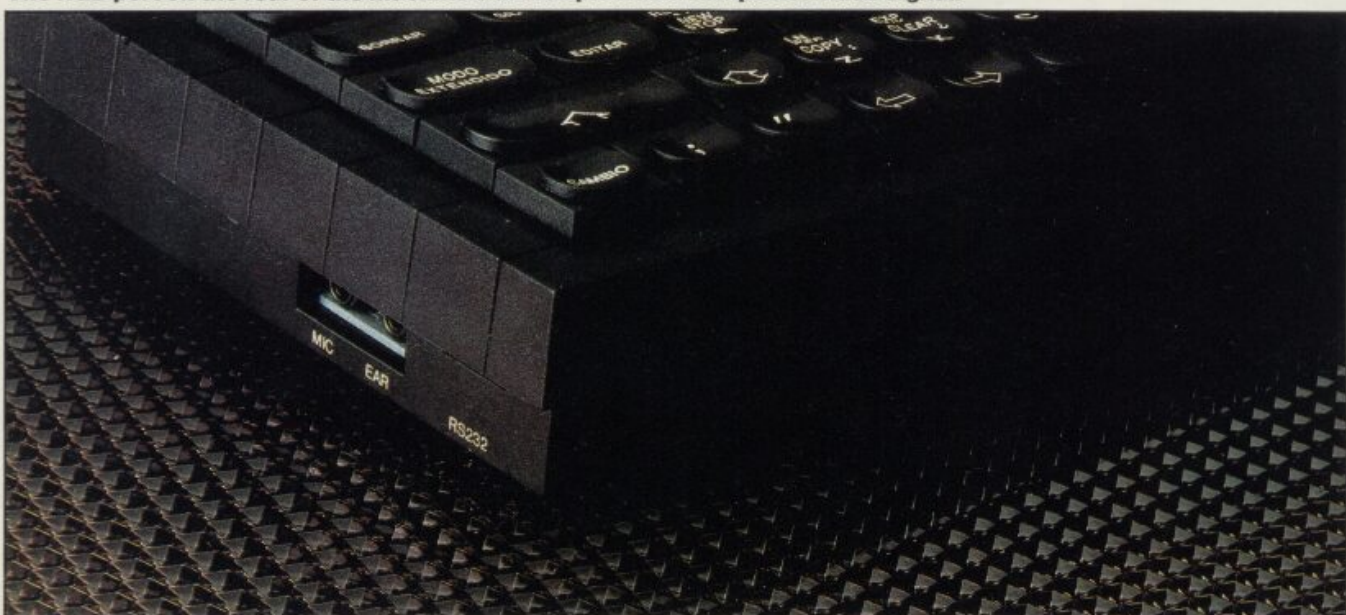
The MIC and EAR ports are now on the left side along with the combined RS232/MIDI interface.
