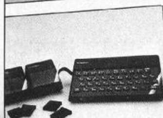
Ordenador Spectrum 48K Micro-Drive + Interface Cintas Micro-Drive
