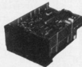
Industry standard interface, compatible with VIDEO GENIE, ATOM, TRS80, BBC COMPUTER, SUPER BRAIN, NASCOM, and lots of others. 3.5 MEGABITS. Unformatted storage capacity, track density 48 TPI. Daisy chain up to 4 drives.
