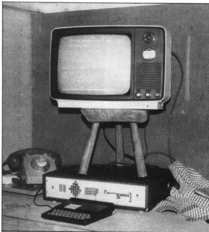
Supported on a milking stool, a TV demonstrates Prestel, conjured up from the phone line by the ZX81 and the adaptor behind it.
