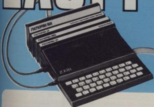
**MEMOPAK Z80 Assembler** This click-in EPROM based pack accepts standard Z80 assembly language mnemonics to allow you to write faster and more compact programs. It has its own ADD, EDIT, LIST, ASSM and QUIT functions, the editor allowing insertion, deletion, automatic line renumbering and error checking. Source code and object code listings can be displayed and printed in decimal or hex format.
