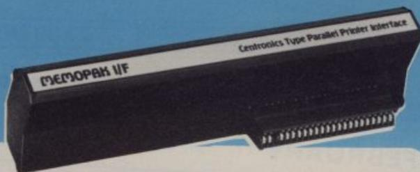
**MEMOPAK Centronics I/F** The BASIC commands LPRINT, LLIST and COPY are used to print on any CENTRONICS type printer. All ASCII characters are generated and translation takes place automatically within the pack. Reverse capitals give lower case. Additional facilities allow high resolution printing. The full capabilities of your printer are now under the control of the ZX81.
