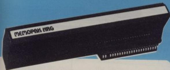
**MEMOPAK HRG** This pack breaks down the constraints imposed by operating at the ZX81 character level and allows high definition displays to be generated. All  $248 \times 192$  individual pixels can be controlled using simple commands, and the built in software enables the user to work interactively at the dot, line, character, block and page levels. Scrolling, flashing and animation are all here.
