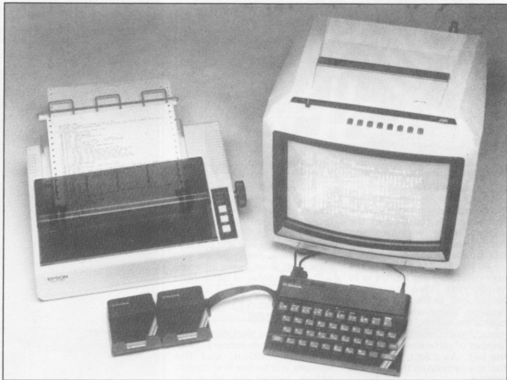
Here you can see the Spectrum connected to an Epson RX 180 printer, a letter quality printer, via the RS232 interface.
