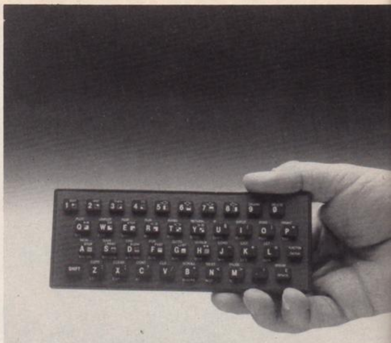
● ZXR Push-Button Keyboard for the ZX81
