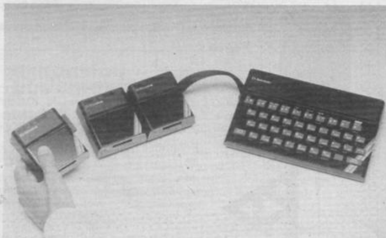
● Up to eight Microdrives can be linked together
