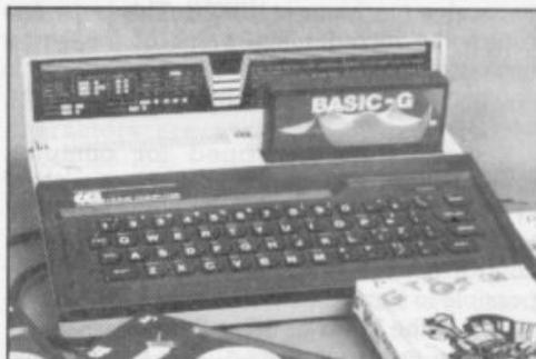
What makes a good machine is a combination of quality and value for money. The Sord M5 (by CGL Home Computers) has broken into the sub £200 market retailing for around £190. For that price you get the basic machine, a rather large external power supply, television lead, Basic I cartridge — a very simple and limited integer Basic — and joypads!
