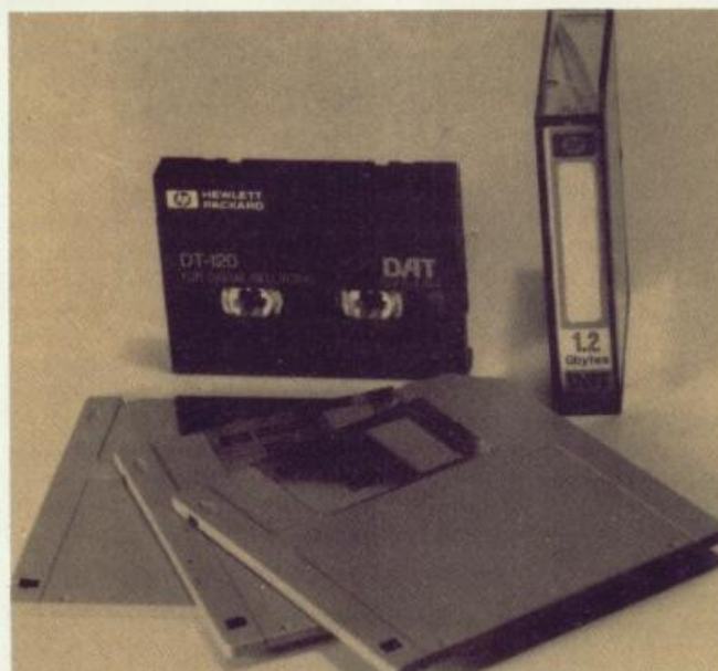
Super cassette, super tape, super price...Hewlett Packard's DAT cassette is half the size of a standard music cassette, but holds 1.2 gigabytes (1258291200 bytes) and can access any file within 20 seconds.
