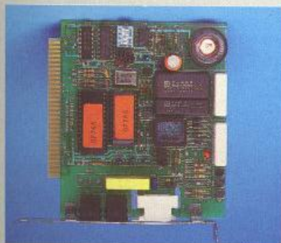
Amstrad 1200 PBS modem card – for the IBM PC
