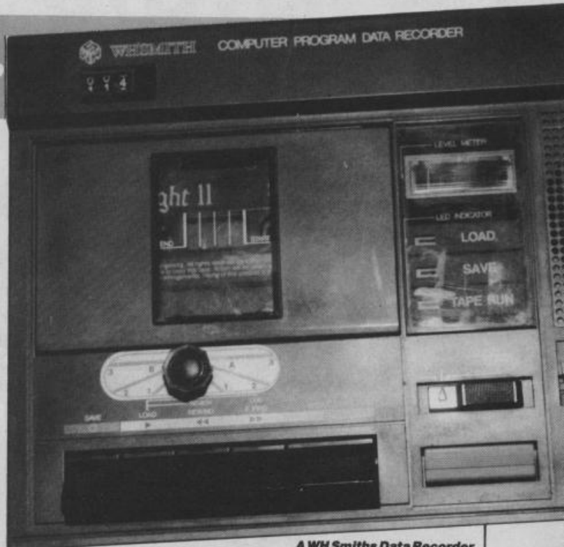
A WH Smiths Data Recorder with the LOAD IT azimuth adjuster
