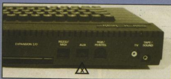
► Behind the scenes: X marks the secret socket on the back of all 128K Spectrums
