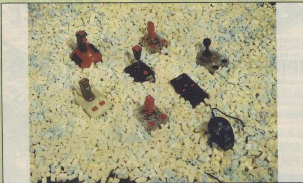
virtues should last some time as the stick has a steel shaft and is fully microswitched – Konix guarantee it for a year. The fire button is also microswitched and is well-placed underneath the player's index finger.
