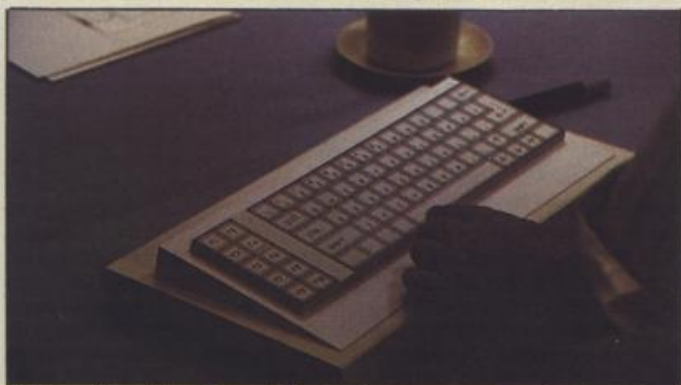
▲ A cardboard mock-up of the designer computer casing
