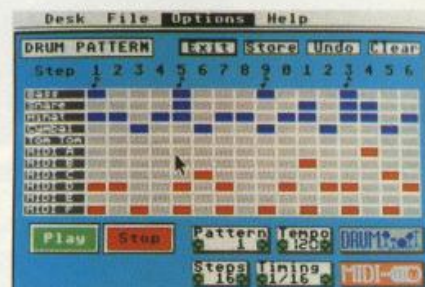
Setting up a drum pattern with FM Melody Maker. The grid rolls from left to right and each filled-in square represents a drum beat on the instrument listed on the left.
