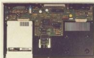
The insides of the machine show just how neatly and carefully it has been designed. The long chip just below the white expansion connector is the Z80B microprocessor, while the square chip at the centre of the PCB is the ASIC – a gate array that connects all the other bits and pieces in the machine.
