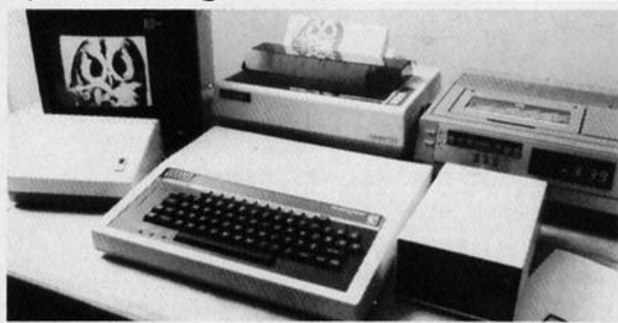
MicroEye — links micro to video recorder
