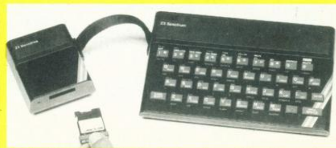
A Microdrive connected, showing how the cartridge is inserted
