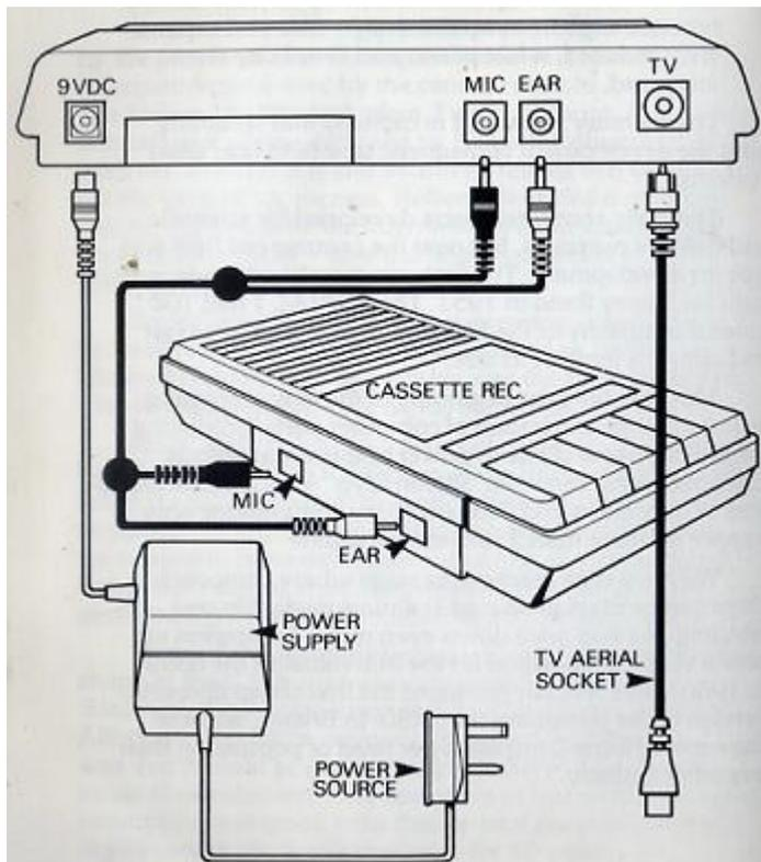
The T.V. should be tuned into Channel 36 (the video channel).
